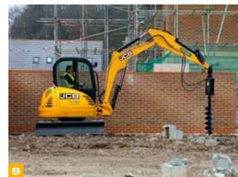
Optimum track footprint for good all-round stability and least-effort spin turning.
